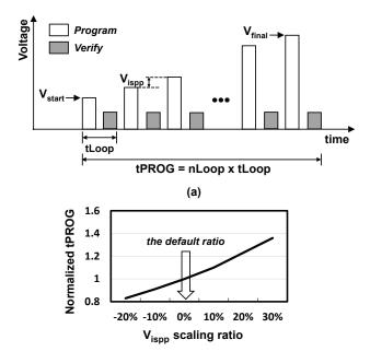
Figure 4: An overview of the ISPP scheme: (a) Key parameters for *tPROG* and (b) Normalized *tPROG* over varying *V*<sub>ispp</sub> scaling ratios
