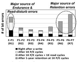
Figure 6: A breakdown of per-state error types on 2x-nm TLC flash.
