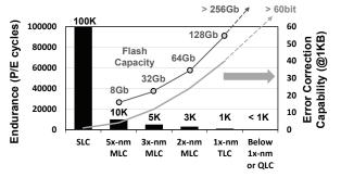
Figure 1: Trends in the flash capacity and flash reliability over advances in flash technologies.
