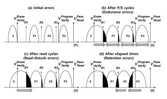
Figure 3: Change patterns in  $V_{th}$  distributions depending on different error types.
