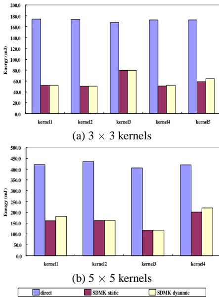
Fig. 5. Energy consumption in the whole Itsy system.
