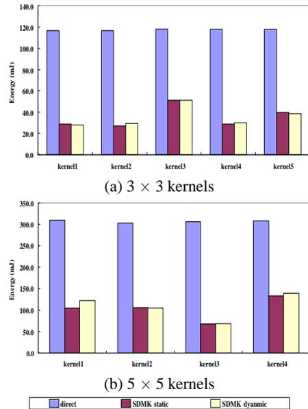
Fig. 4. Energy consumption in the StrongARM processor core.
